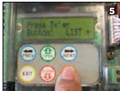
5 Press the orange 'SET' button once, the display should show the above message and the unit will start beeping.
