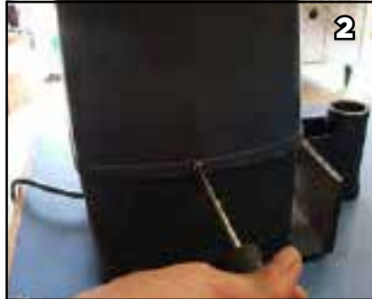
2 To remove the cover locate the two cover screw, one located on each side, and unscrew them.
