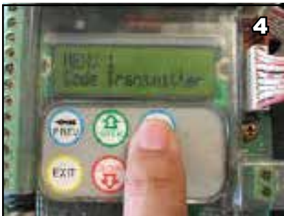
4 Press the blue 'NEXT' button once till the display shows 'Code Transmitter'.
