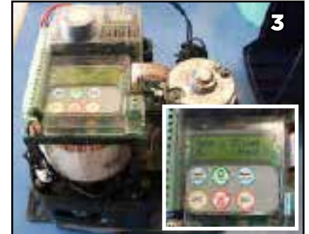
3 Lift off the cover to reveal the receiver board and digital display.
