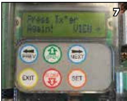
7 The display will show the following message and the unit will start beeping faster.
