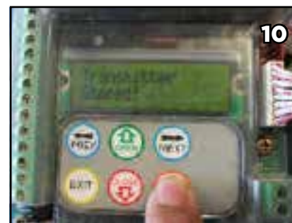
10 The display will show the message 'Transmitter Stored!'. This means your new remote was successfully programmed. Replace cover and test at the motor to confirm.
