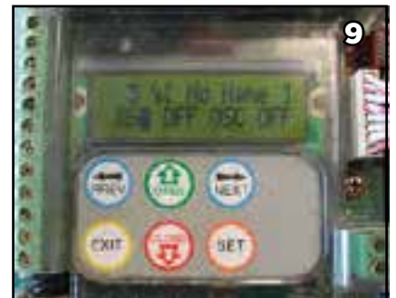
9 The display will now show the above message. Press the 'SET' button once.
